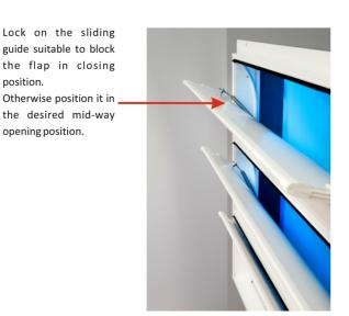
Each flap has an easily adjustable counterweight which allows the increasing or decreasing of the negative pressure required for flap opening, simply by screwing or tightening the two nylon wing nuts.
