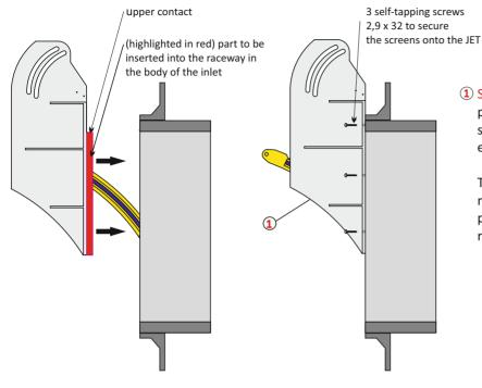
1 SIDE SCREEN= Right and left side screens are used to prevent the incoming air flow from deviating to the side. These screens include a space in which you can eventually house an adjustable deflector.
